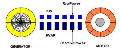
The figure below shows the results of installing a capacitor near the same motor to supply the magnetising current required to operate it. The total current requirement has been reduced to the value of the useful current only, thus either reducing power cost or permitting the use of more electrical equipment on the same circuit.
