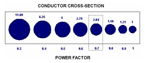
Practically speaking, when an installation uses its rated power capacity, the distribution cables within the installation are rapidly loaded to their full carrying capacity if the power factor decreases. Most often, as the need for energy in an installation expands, the first reaction is to double the distribution system although it would be less expensive to perform a correction of power factor on each load or group of loads.
