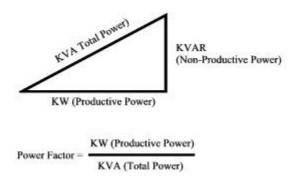
The cosine of the phase angle  $\theta$  between the KVA and the KW components represents the power factor of the load. KVAR represents the non-productive reactive power and  $\theta$  is lagging phase angle.
